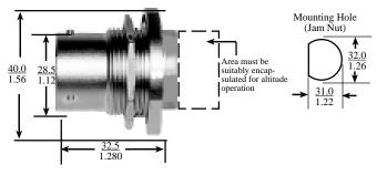
**P/N 167-8666** Sealed. Rear mount/Jam nut receptacle Insulator: Plastic
