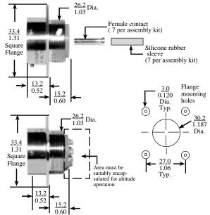
P/N 178-8741 Kit. Front Mount/Box Flange (shown top) Plastic insulator and loose contacts. 7 female contacts
