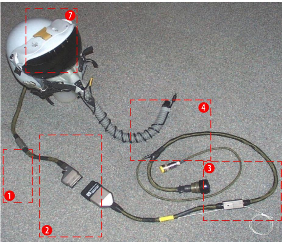
① The Helmet Release Connector (HRC) permits the helmet to be shed in the event of inadvertent helmet loss during ejection.
